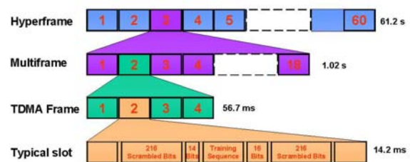
Figure 1 - Air Interface - TDMA illustrated
